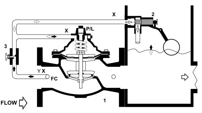
Flow Direction Shown: Flow Under the Seat Optional "R" Flow Over the Seat: 110-10R/1110-10R
