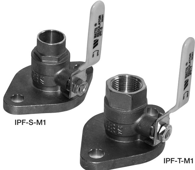
\*This valve is designed to be soft soldered into lines without disassembly, using a low temperature solder to 420°F (216°C). Higher temperature solders may damage the seat material.
